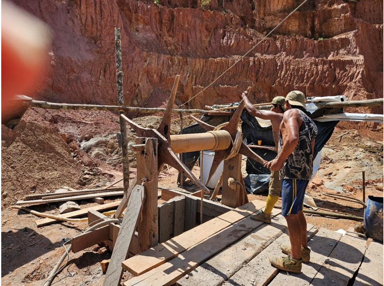
Figure. 21. New shaft by Brazilians Jons trend. Quartz brought up by bucket cut from ½ fuel barrel. Photo by author, 2024.
