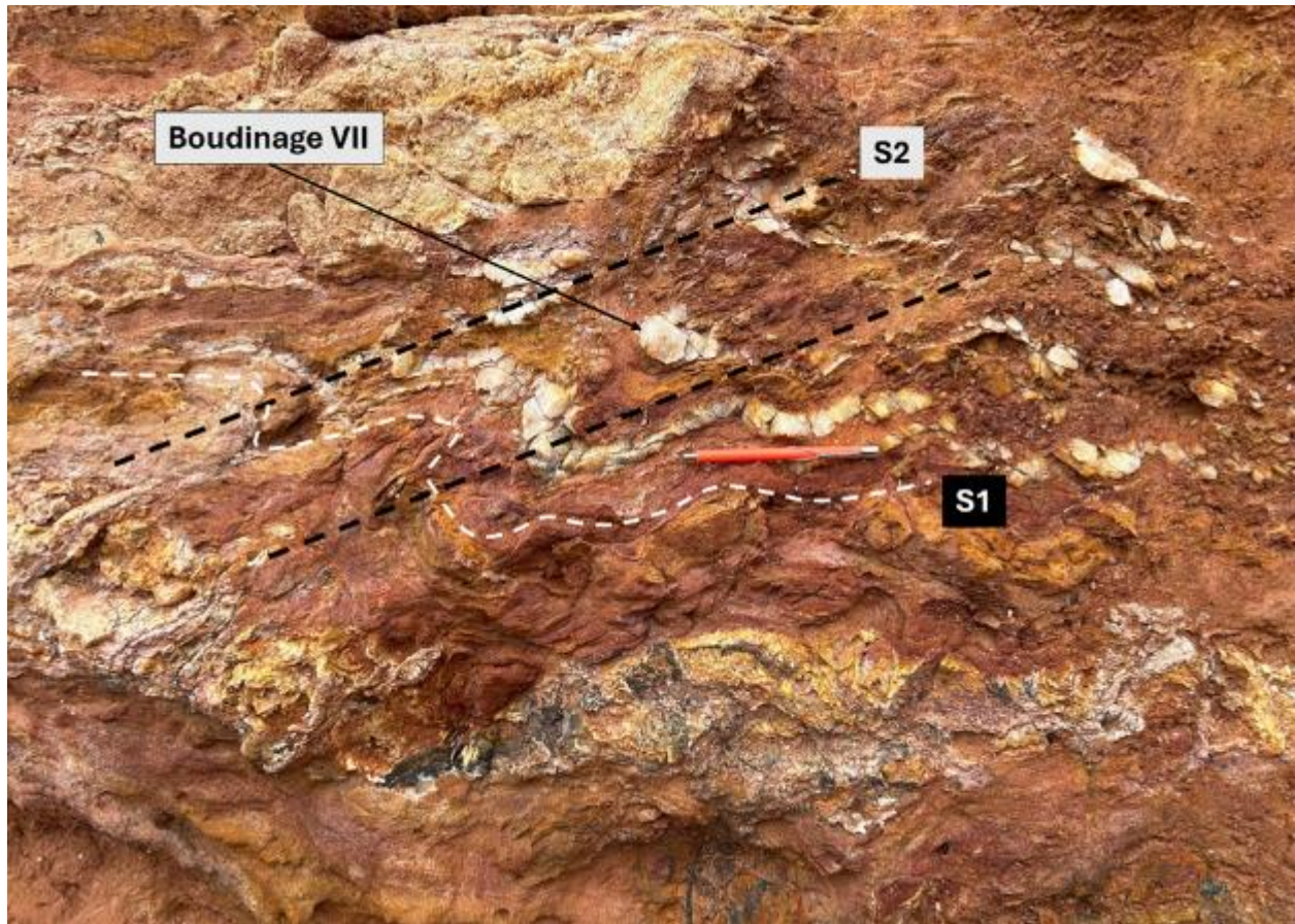
Figure 7.7 Folded S1 and S1-parallel boudinaged quartz veins in the Howler prospect. S2 axial planar cleavage Intersection lineation and fold axes to veins @ 10-140. Photo by Miata.
