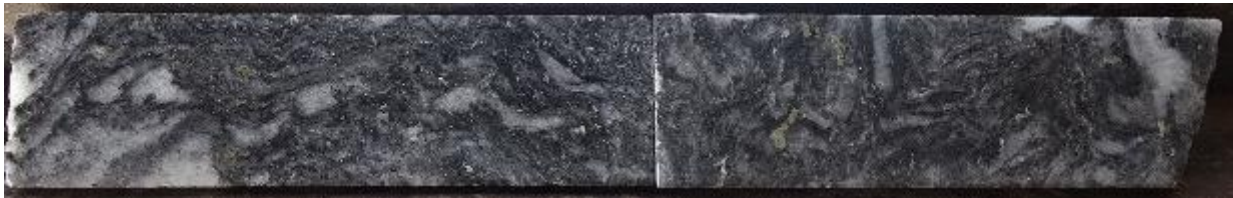
Figure 10.11. Hole 25DDH-SEL-033 101.50 m, 15.55g/t Au, folded and boudinaged quartz veins
