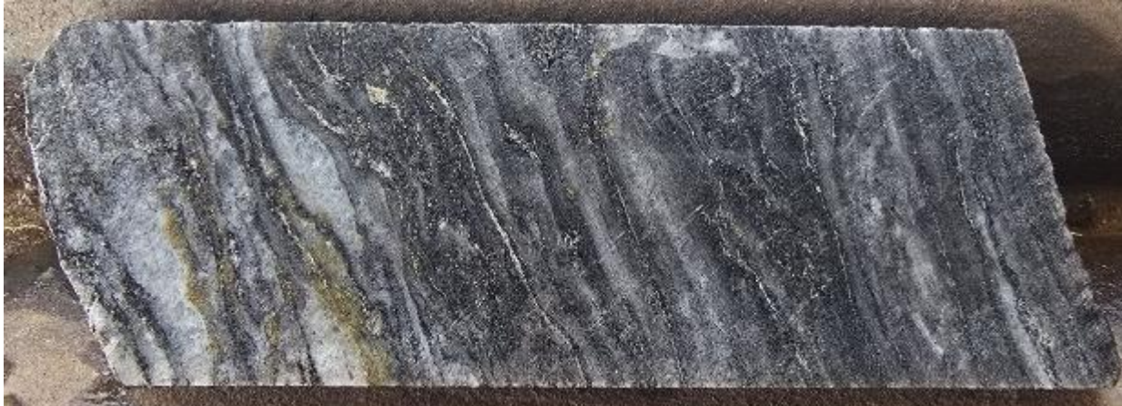
Figure 10.10. Hole 25 DDH-SEL-033 at 095.00 m, 2g/t Au, in sinistral sheared layered quartz.
