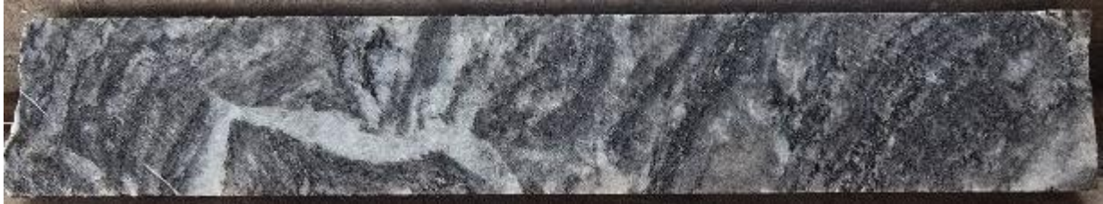
Figure 10.9. Hole 25DDH-SEL-033 at 092.20 m, 10.5g/t Au, with banded quartz veining parallel to S1 in folded biotite schist.
